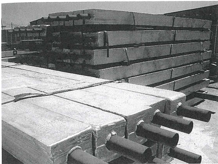
FIGURE 9.5.8 These aluminium sacrificial anodes are attached to the underwater steel structures of offshore gas platforms to protect them against corrosion.
